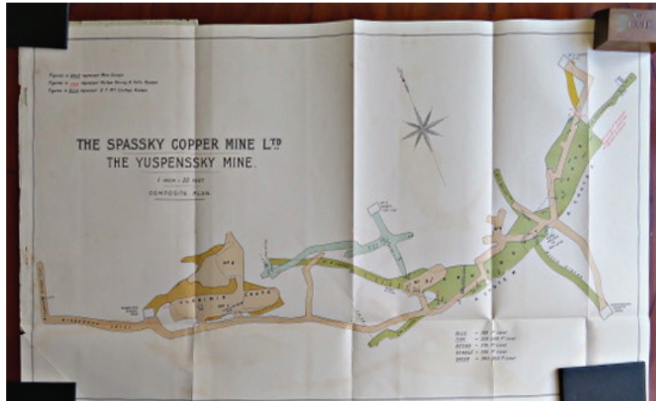
Fell's plan of the Uspensky Mine; the weight on the top right corner, is a small ingot of copper, stamped '1905 F' (for Fell)
